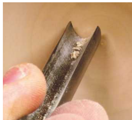
▲ Pic.5 This tool is my first choice for finishing off the centre of the bowl. The wood in the middle is not revolving very quickly so you will need to slow the feed speed down to almost nothing when you reach the middle
